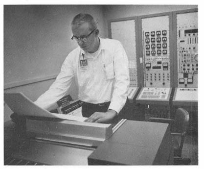
AEROSPACE GROUND EQUIPMENT designed by Section 7432-1 performs 50,000 individual tests in seconds on the satellite's logics systems. John R. Phelan (7432-1) checks computer read-out from the AGE. The equipment is programmed to pinpoint failure in any of the thousands of tiny components of the logics system undergoing performance tests.
